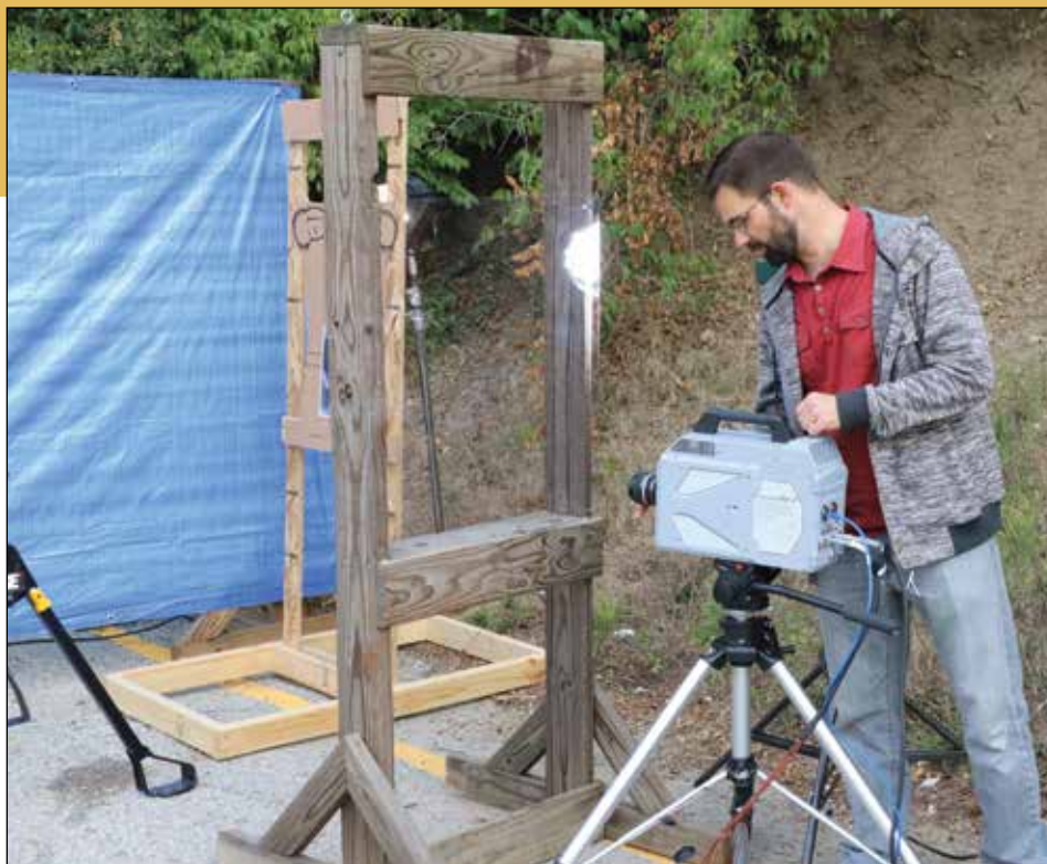
Travis Ross, the manager of the Visualization Lab, adjusts the high-speed video camera he used to record the point-of-impact as three different types of ammunition penetrated various barriers. It was part of a project with the sniper unit of the Champaign County Metropolitan Emergency Tactical Response Operations (METRO).
