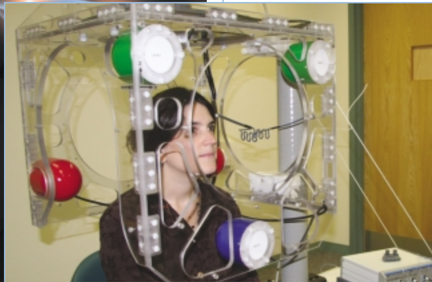
Beckman Fellow Sarah Brown-Schmidt tries out the new AG500 3-D articulograph installed at linguistics researcher Chilin Shih's laboratory at the Beckman Institute. The rare electromagnetic articulometer, called EMA, is used to measure physical movements during speech production.
